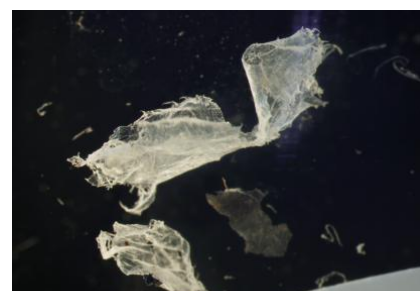
Figure 7. Films found at Lobith (Rhine river), sample L16. Scale bar=500 µm
