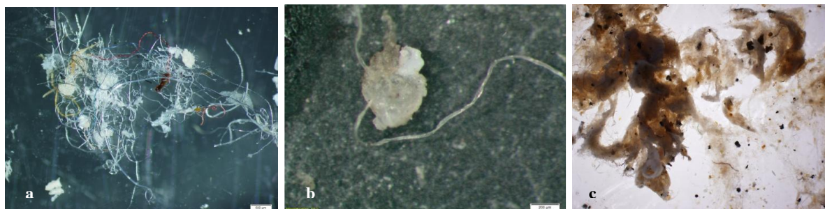
Figure 35. Fibres were regularly observed and they occasionally caused hindrance for microscopic study, such as (a) A clew of polymeric fibres found in the Rhine River (Bad Honnef) holding target MPs. Scale bar = 0.5 mm. (b) A scrub particle and a polymeric fibre molted together. Scale bar = 0.2 mm. Picture taken in pilot phase after HNO 3 digestion. (c) Lumps of (suggested) cotton fibres found in Meuse river (sample E14, 0.250-
